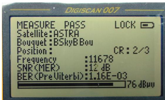
Pressing the **Enter** key enables the meter to measure the chosen frequency (transponder). Pressing **Enter** again will return the Digiscan to the spectrum display
