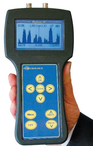
Unlike most low cost satellite meters the Digiscan displays the frequency spectrum of the satellite band. Using the spectrum gives a great deal of information. Here we take a closer look at what the display is telling us:
