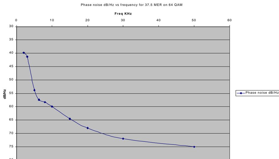
The graph shows the maximum phase noise in dB/Hz to give a MER of 37.5 dB. From these results we made a template which could be placed over our plots of oscillator noise to check their performance.
