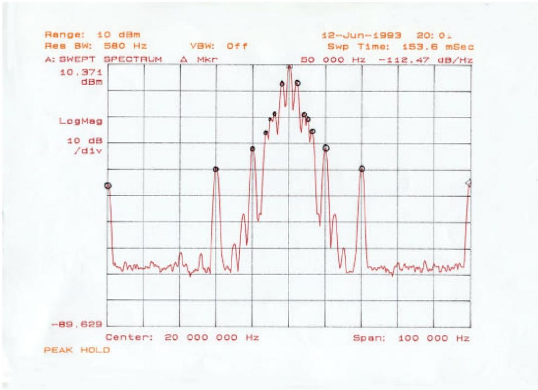
A Hewlett Packard HP3588A spectrum analyser which has an exceptional specification including a resolution bandwidth down to 1.1Hz and a phase noise of better than  $-115$  dB/Hz was used to monitor the phase noise on the second local oscillator and this produced the graph shown. I emphasise the quality of the spectrum analyser as most spectrum analysers have more phase noise than the oscillators we were measuring!
