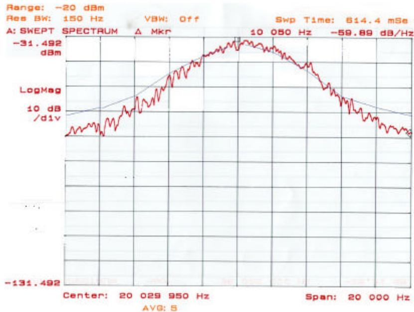
The plot above shows the original oscillator design, the margin is zero.
