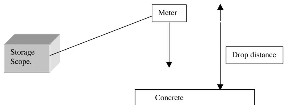
The meter in its carrying case was dropped onto concrete from an increasing height and the storage scope recorded the g force registered by the accelerometers. After each drop the unit was checked for damage. The drops were repeated 2 times in both end-on and face down mode and the results are the highest recorded g at each height.
