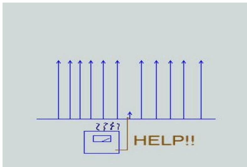
The noise floor measurement made by the test instrument is in the presence of many signals often with peak amplitude 60 dB greater than the signal to be measured. These high levels can cause overloading of the signal level meter or spectrum analyser used to make the signal to noise measurement. The noise floor may contain beat products from analogue vision carriers that are higher than the noise level.
