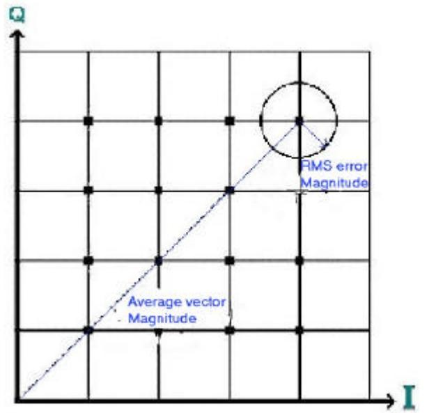
The above diagram shows one quarter or quadrant of a constellation display of a 64 QAM signal, from the following formulae MER can be calculated.
