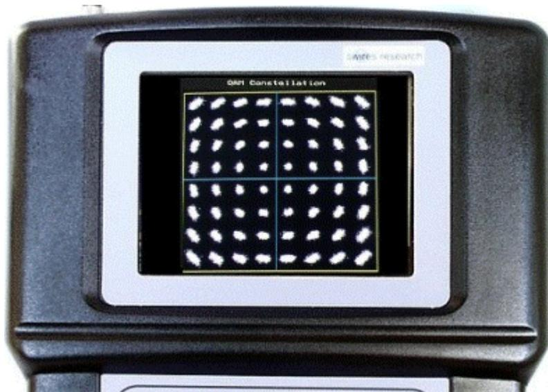
The picture above shows the effect of phase noise as the rounding effect this is most noticeable at the corners of the display.
