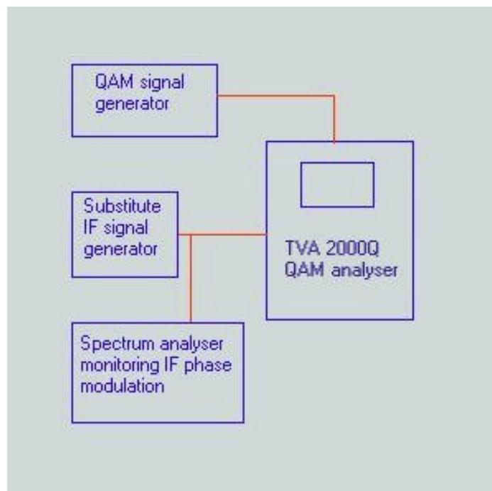
A reading of the MER was taken using the QAM analyser under test. This gave a MER of 37.5 dB.
