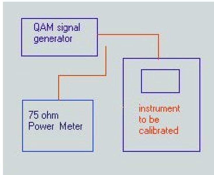
Take a single digital modulator and feed the signal into a high quality calibrated power meter.
