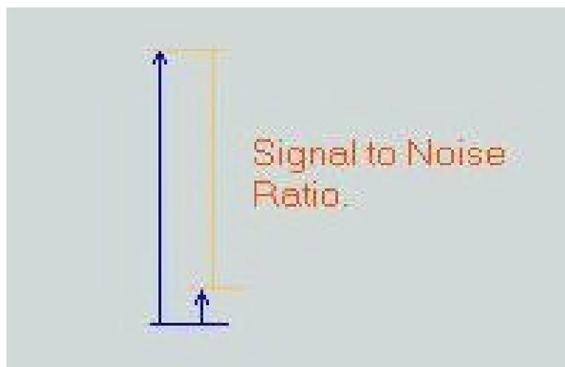
Nice and simple, measure the level of the desired signal, then move to a frequency away from the signal and measure the level of the noise floor. The difference in dB's is the signal to noise ratio.
