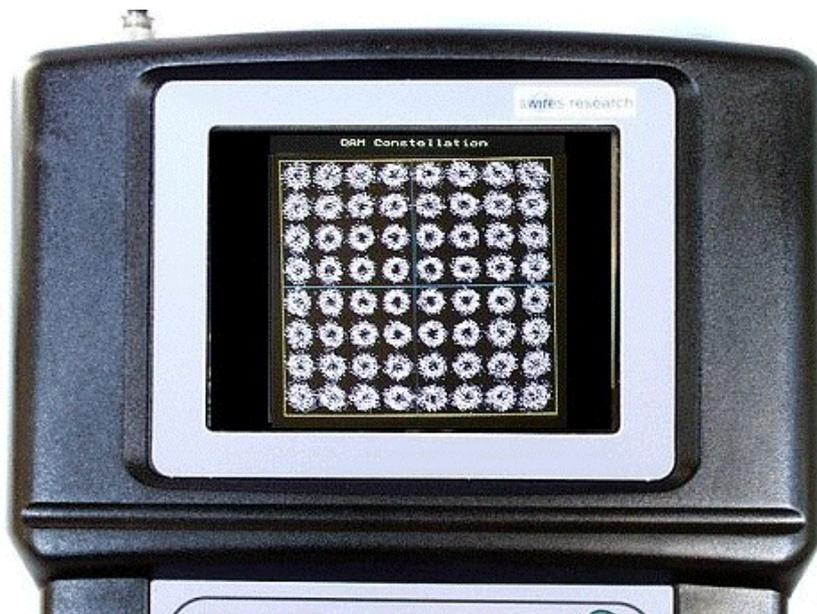
This 'polo mint effect' is caused by a single carrier interference, in channel approximately 25 dB down on the digital signal.
