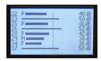
Each channel (up to 8) is represented by a horizontal bar.
