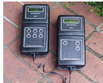
Special interface lead -plugged between Charge sockets.
