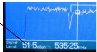
The unit of measurement can be either dB $\mu$ V or dBmV selected in the Set up Menu. (Menu , Set up Menu , set display to dB $\mu$ V / dBmV).
